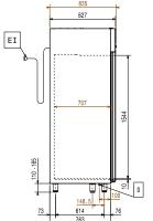
Electrical inlet (power) Refrigerant Inlet RΙ Refrigerant Outlet
